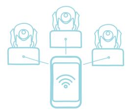
With the Stogger FRD-e application, you can easily control multiple FRD-e's. Next to the basic settings, also advanced settings such as PEEP and plateau time can be set. The application eliminates the need to be near to a FRD-e, greatly reducing the potential infection risk a doctor or a nurse faces.
