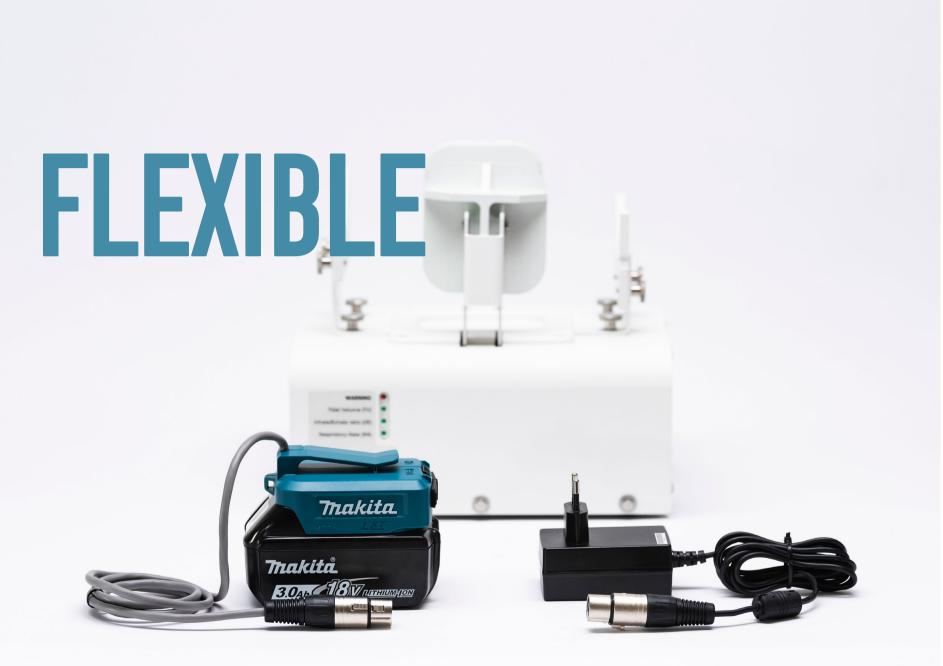
The FRD-e can be powered using a multitude of power sources. The device has two power connectors, each suitable for an independent power supply. Typically one connector is paired with an external 24Vdc power supply. As a backup the second power terminal can be hooked up to an external battery. This can be any power supply ranging from 18-24 Vdc. As an example: a typical 18V 5Ah cordless drill battery can power the device for up to 10 hrs\*.
